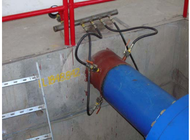
Figure 2.2 - Pressure taps connected through separate connecting pipes to box-type manifold
