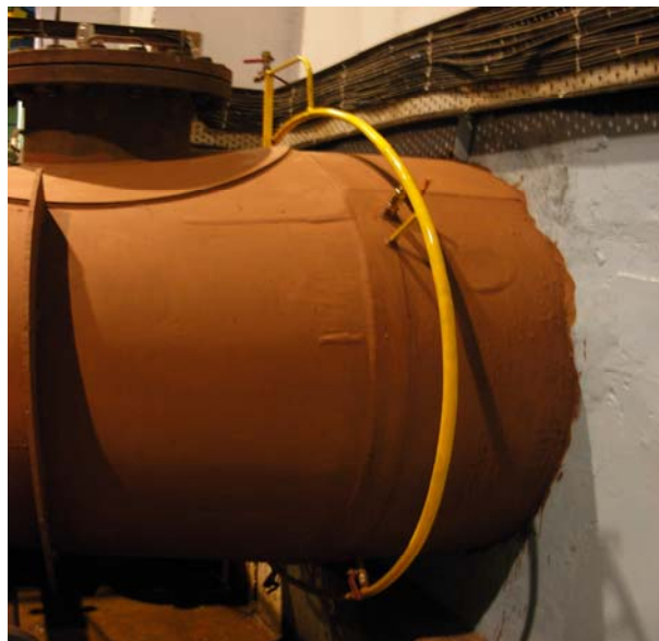
Figure 2.3 - Pressure taps connected through ring-type manifold to pressure gauge
