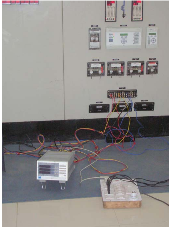
Figure 9.3 – A reference meter connected at TTB without opening the control panel
