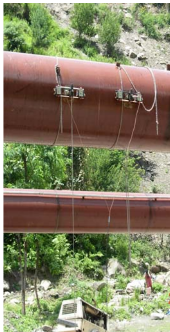
Figure 7.5 – Transducers of the UTTF clamped on a penstock in reflection mode
