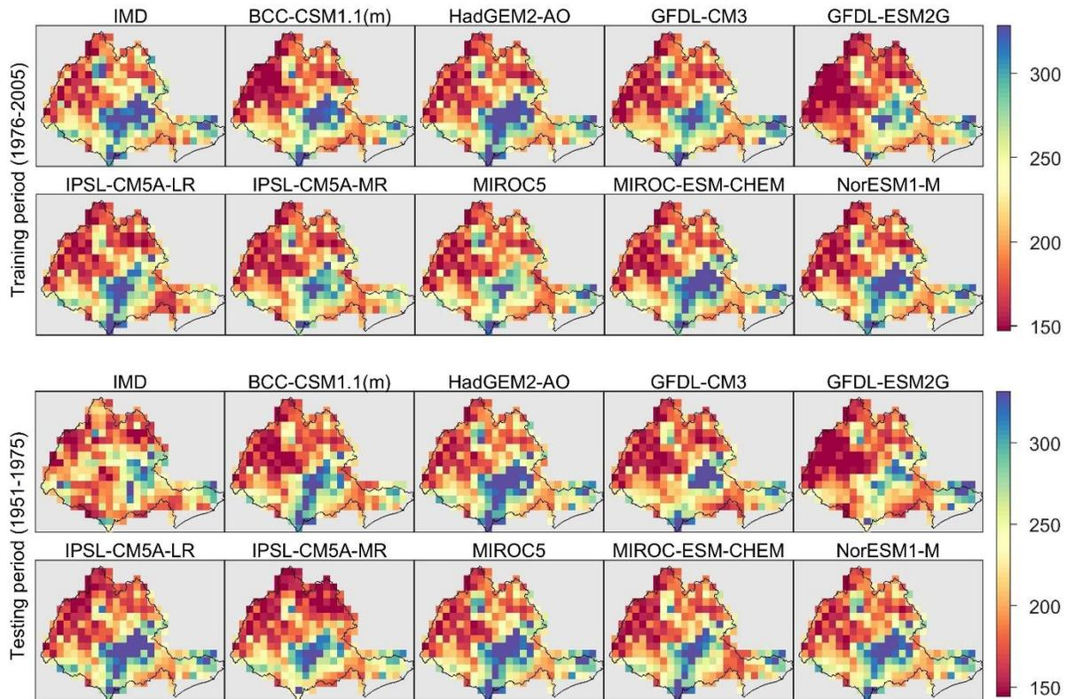
**Fig. 4** Spatial maps of 50 year return period rainfall for IMD and bias-corrected GCMs using monthly hybrid approach. Color bar in the right shows rainfall depth in mm.
