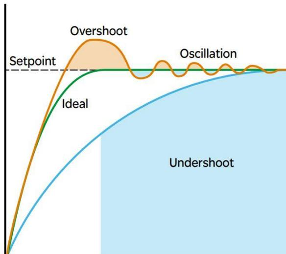
Actuator Output =  $K_p * (\text{distance from goal}) + K_d * (\text{change in error}) + K_i * (\text{accumulative error})$
