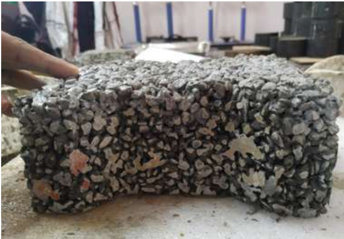
Figure 11 A photo of PerVIOUS Paver Block which allows groundwater recharge and reduces waterlogging and urban heat island effect
