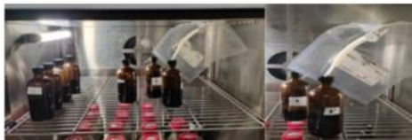
AD bottles with tedlar bags inside the cabinet at temperature 35°C
